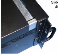
Slide the enclosure cover backward to disengage it from the guides at the
